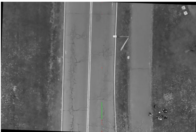
Fig. 12. A false positive. Here, part of the road is cracked significantly more than other sections of the road, so the cracks are assessed to be cars.
