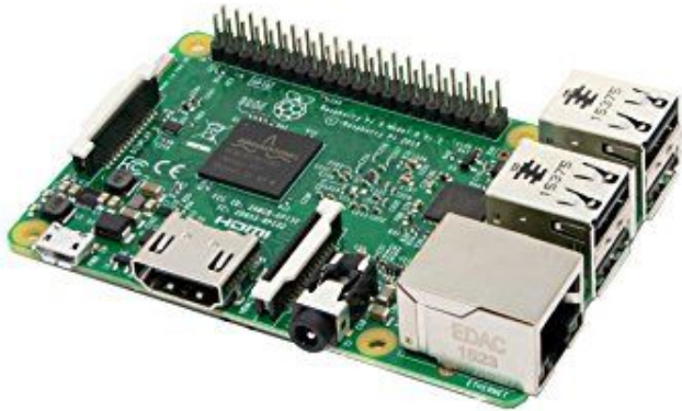
Fig 2. Raspberry Pi, compact computer used for educational purposes
