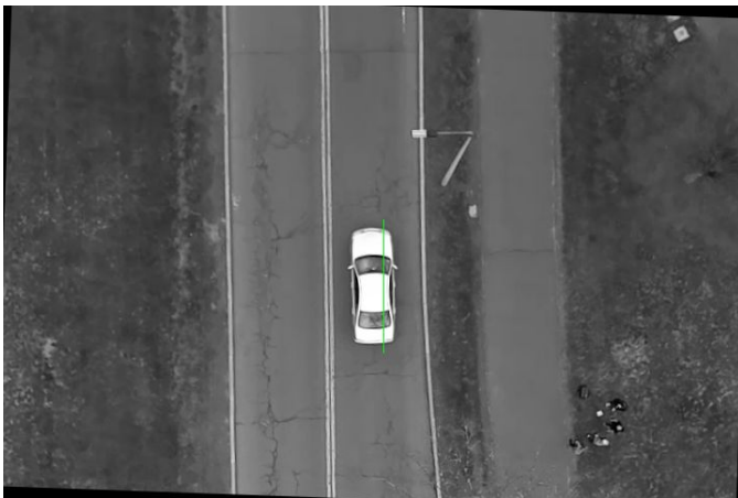
Fig. 11. A successfully identified car, shown here as green pixels
